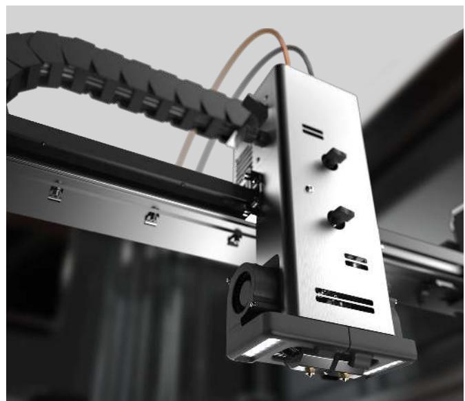
The STUDIO has a unique dual extruder equipped with two 0.6 mm hot ends, which has been optimized for both speed and precision. The second hot end retracts to enable clean dual extrusion prints. The STUDIO's extruder enables printing with a layer height of 0.1 mm
